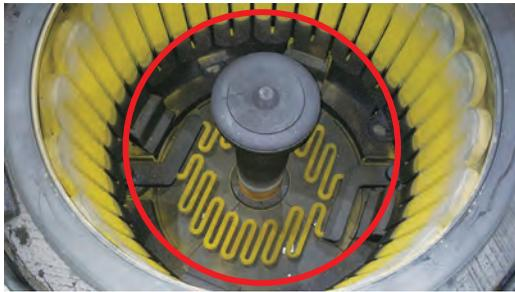
·Thermal components for Puller were changed to Low Power Hot Zone (LPHZ Type).
